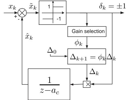
Fig. 6. Adaptive coding scheme (only the encoder structure is depicted). The figure shows the case of one-dimensional systems. The selection gain block toggles the value of  $\phi_k$  according to Equation (24).
