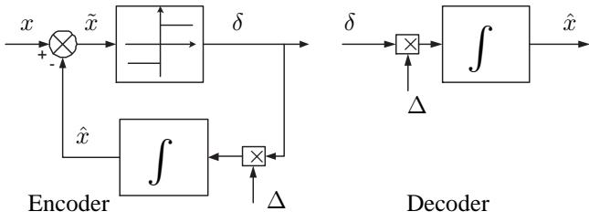
Fig. 4. Block diagram of standard continuous-time version of the  $\Delta$ -M coding scheme. The encoder  $\Phi_E$  is depicted at the left, where the decoder  $\Phi_D$  is shown at the right. For  $n > 1$ ,  $\delta$  is defined as  $\delta = [\delta^1, \delta^2, \dots, \delta^n]^T$ , with  $\delta^i \in -1, 1$ .
