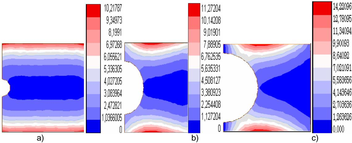
Fig. 7. Contour of the levels of shear adhesive stresses for different notch radius
