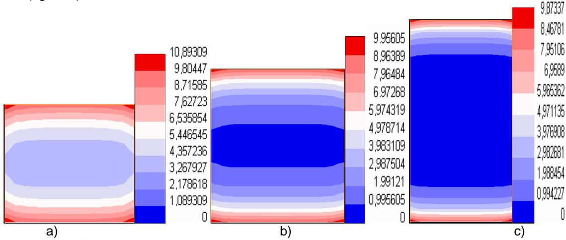
Fig. 6: Contour of the levels of shear adhesive stresses for different adhesive length
