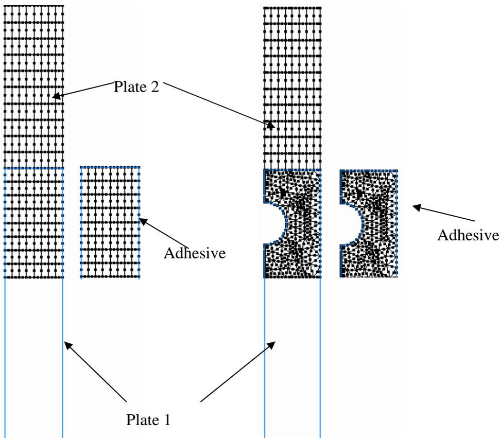
Fig. 2: Typical mesh model of one aluminum plate, a) no notch, b) with notch.
