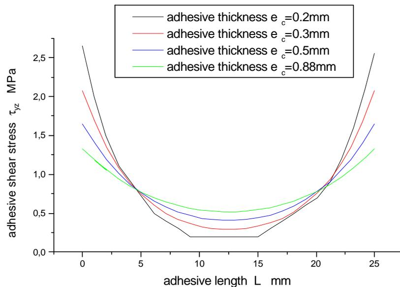
Fig. 3: Distribution of adhesive shear stress according to the length of adhesive for different adhesive thicknesses (without notch and with aluminum plates, applied stress =35 MPa).
