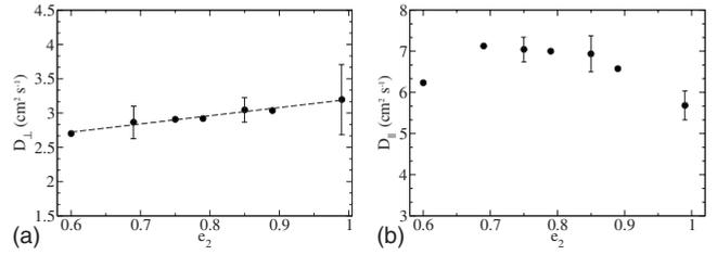
FIG. 16. Evolution of (a)  $D_{\perp}$  and (b)  $D_{\parallel}$  versus  $e_2$  for  $N=2000$ ,  $D/d=10$ ,  $D=20$  mm,  $H/D=14$ , and  $e_1=0.84$ . An unweighted linear least-squares regression is represented in case (a).
