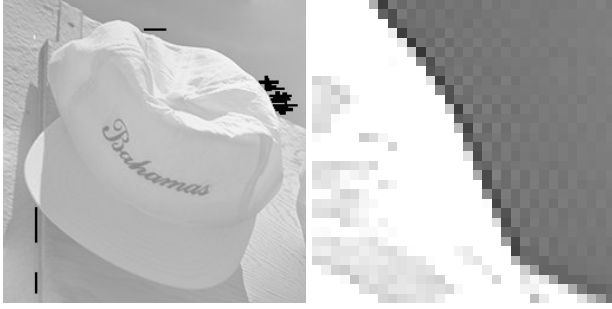
Fig. 3. The ‘caps’ image from the Live database is not well-sampled: ringing is detected (black zones on the left image) after an horizontal translation of 0.5 pixel, especially near the top-right corner of the cap. The image on the right zooms on this part, with contrast magnification and no detection marked.
