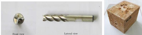
Fig. 4. The drill bit (left), and the cedar wood block specimen (right)
