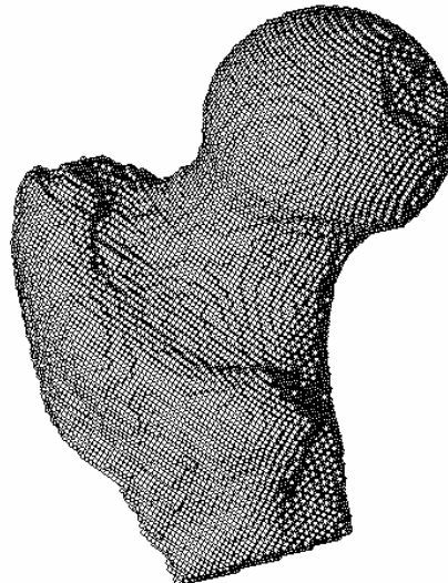
Figure 2. (a) Voxel based mesh model of the first femur.
