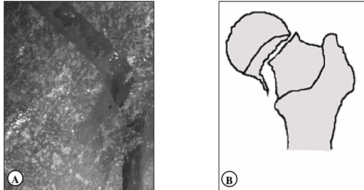
Fig. 3. Rupture profiles obtained. (A) Rupture line of femur-1 observed by photo acquisition system. (B) Schema of femur-1, femur-2 and femur-3 rupture profile.
