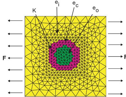
Fig. 22. Example 2. Plate with a random hole in tension; X-SFEM mesh with three element groups: surely inside the domain ( $e_i$ ), possibly cut by the boundary of the hole ( $e_c$ ) and surely outside the domain ( $e_o$ ).
