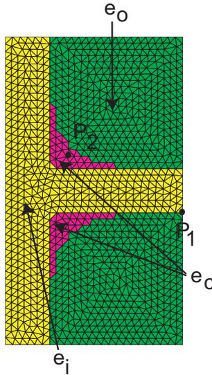
Fig. 28. Example 3. X-SFEM mesh with three element groups: surely inside the domain ( $e_i$ ), possibly cut by the boundary ( $e_c$ ) and surely outside the domain ( $e_o$ ).
