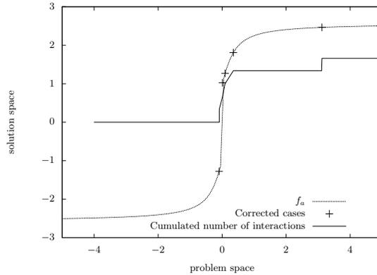
**Fig. 5.** Distribution of the corrected cases around a discontinuity (with  $\varepsilon = 0.2$ ). The dotted line represents the function to approximate, the crosses are the solved cases that have required a correction from the oracle and the plain line represents the accumulation of the number of interactions with the oracle.
