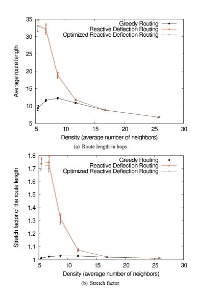
Figure 6: Route length under different routing schemes for UDG.
