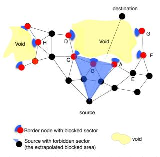
Figure 4: Method for locally detecting the border of a void.
