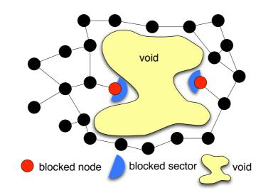
Figure 1: Blocked nodes in greedy geographical routing.
