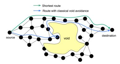
Figure 3: The increase of route length when surrounding a void.
