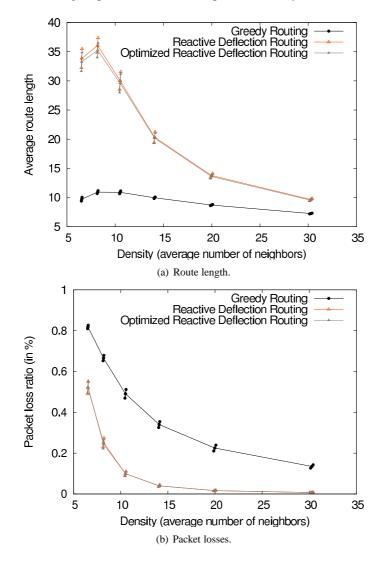
Figure 7: Performances of different routing schemes for a proxi-graph with one central void.
