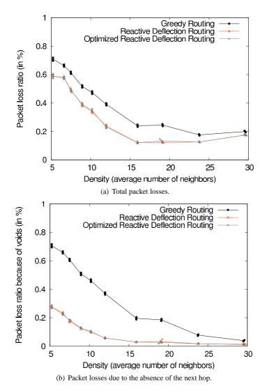
Figure 8: Packet loss ratio under different routing schemes in ns2.
