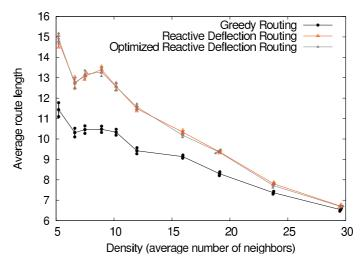
Figure 9: Route length under different routing schemes in ns2.
