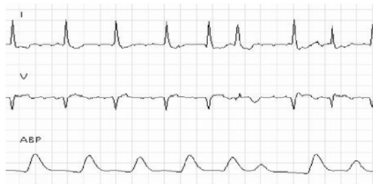
Figure 1 Multisource data: lead I and V of an electrocardiogram and an arterial blood pressure channel
