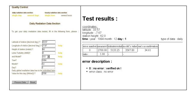
Figure 1. Screening daily irradiation. Left) the form for screening a single day. Right) the screening results.
