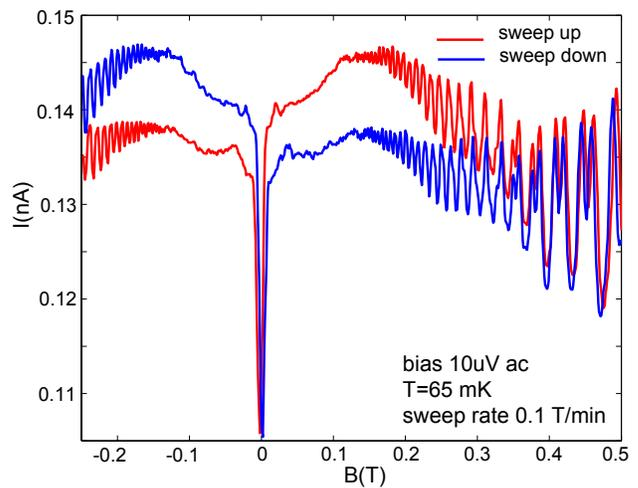
FIG. 1: Current through a pair of ohmic contacts at  $T=65$  mK as a function of magnetic field at fixed ac bias of  $10\mu\text{V}$  and  $B$ -sweep rate 0.1T/min. The red trace correspond to  $B$ -field up-sweeps and the blue trace to a down-sweep. As the  $B$ -field approaches a value around 0.5 T, the hysteresis disappears.
