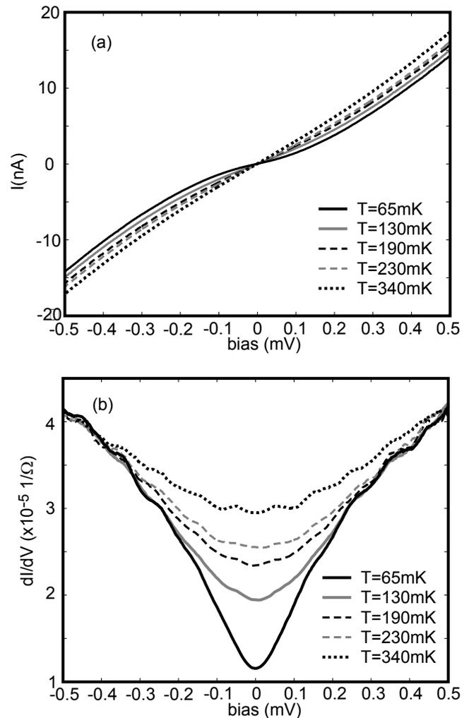
FIG. 3: (a) Temperature dependence of the  $I$ - $V$  characteristics of In/Zn/Au ohmic contacts at  $B=0$ . (b) Temperature dependence of the differential conductance  $dI/dV$ , obtained by numerical differentiation of the  $I$ - $V$  traces shown in (a).
