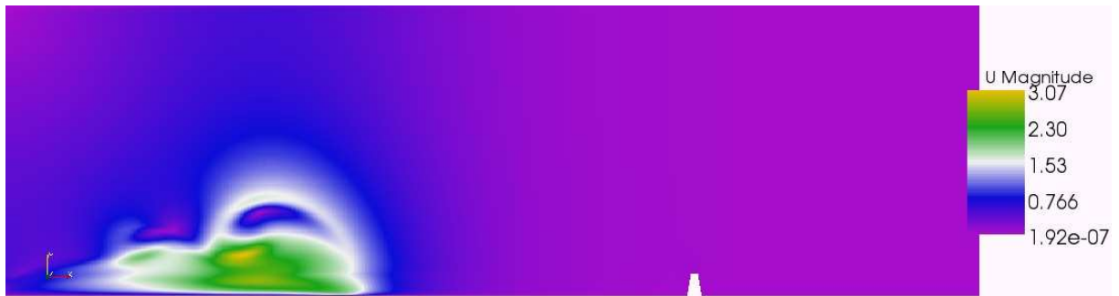
FIGURE 8. Velocity field magnitude at t = 25 s. The color scale ranges from 0 m/s to the maximum value 3.07 m/s.
