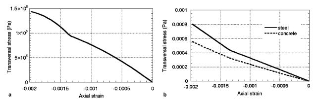
Fig. 13. Transverse behaviour using the elastic damage model: (a) evolution of the transverse stress as a function of the axial strain; (b) evolution of the concrete and steel transverse strains as function of the axial strain.
