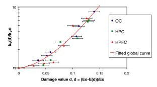
Fig. 1. Experimental relation between damage and permeability.  $k_{v0}$  and  $k_v$  are the intrinsic permeabilities of the initial and damaged material, respectively, [36]. OC = ordinary concrete, HPC = high performance concrete, HPFC = high performance fiber reinforced concrete.
