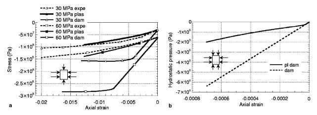
Fig. 9. Comparison between elastic damage and elastic plastic damage constitutive laws: (a) triaxial tests with increasing confinement. Axial stress-strain curves for high hydrostatic pressures; comparison between the elastic damage model (dam) and the elastic plastic damage formulation (plas); (b) hydrostatic confinement. Comparison between elastic damage model (pl dam) and elastic damage constitutive law (dam).
