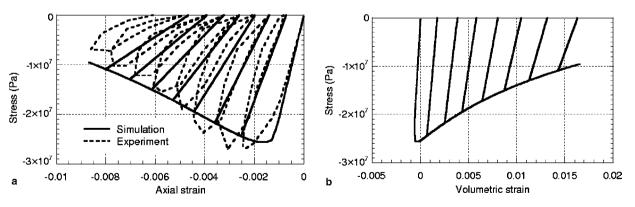
Fig. 7. Simulation of a cyclic compression test [44]. Elastic plastic damage response.
