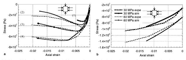
Fig. 8. Triaxial test with increasing confinement. (a) Axial stress-strain curves for low hydrostatic pressures. Straight lines (black markers) correspond to simulation, dotted lines (white markers) to experiment (1) 0 MPa, (2) 1.5 MPa, (3) 4.5 MPa, (4) 9 MPa. (b) Axial stress-strain curves for high hydrostatic pressures.
