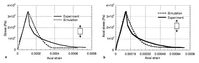
Fig. 5. Simulation of a uniaxial tension test [13]: (a) elastic plastic damage formulation; (b) elastic damage model.
