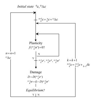
Fig. 4. General algorithm for the elastic plastic damage model.
