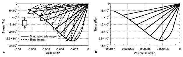
Fig. 6. Simulation of a cyclic compression test [44]. Elastic damage response.
