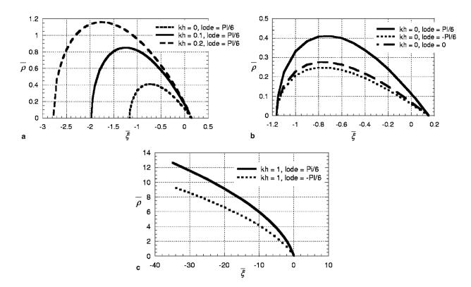
Fig. 3. (a) Evolution of the yield surface with the hardening parameter for a constant lode angle  $(\frac{\pi}{6})$ , (b) evolution of the yield surface with the lode angle for a fixed hardening parameter and (c) failure surfaces for two lode angles.
