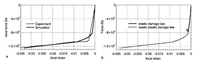
Fig. 11. Simulation of a CFT: (a) evolution of the axial force as a function of the axial strain. Comparison between the elastic damage formulation and the experiment; (b) comparison between the elastic plastic damage and the elastic damage models.
