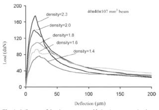
Fig. 4 - Influence of density on structural behavior, average load-deflection curves for different material density on  $40 \times 40 \times 107~\text{mm}^3$  beams.
