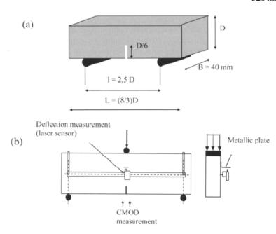
Fig. 2 - (a) Description of mortar samples; (b) Description of instrumentation for the bending tests.
