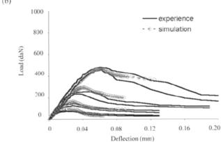
Fig. 11 - Model calibration for mortar beams with material density 2.3 (a) and 1.4 (b).
