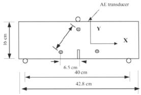
Fig. 7 - Specimen geometry and AE transducers placement.
