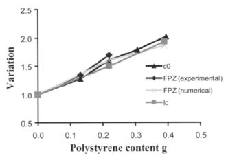
Fig. 13 - Evolution of d<sub>0</sub>, FPZ (experimental), FPZ (numerical) and internal length with polystyrene content.
