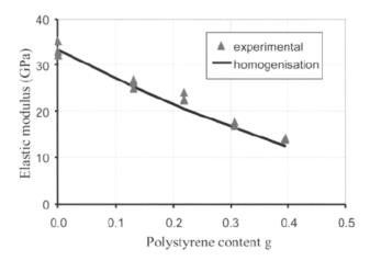
Fig. 3 - Variation of elastic modulus with polystyrene content.
