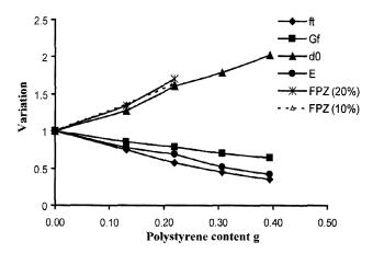
Fig. 10 - Evolution of mechanical properties with polystyrene content.
