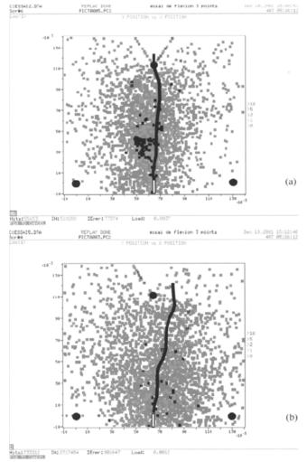
Fig. 8 - Cumulative location of AE events: (a) material density 2.3; (b) material density 1.8.
