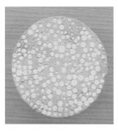
Fig. 1 - Distribution of polystyrene beads in 1.4 density mixture.
