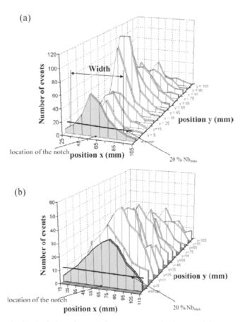
Fig. 9 - Evolution of cumulative events per grid: (a) material density 2.3; (b) material density 1.8.
