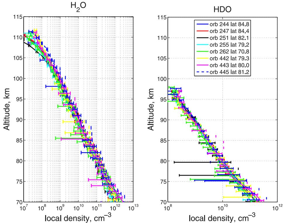
**Figure 10.** Vertical distributions of the H<sub>2</sub>O and HDO local density for eight orbits: five consecutive orbits from MTP09 (from 19 December 2006 to 10 January 2007) and three consecutive orbits from MTP016 (from 1 July 2007 to 27 July 2007), where MTP is the medium term plan. The conditions of observations are listed in Table 1.
