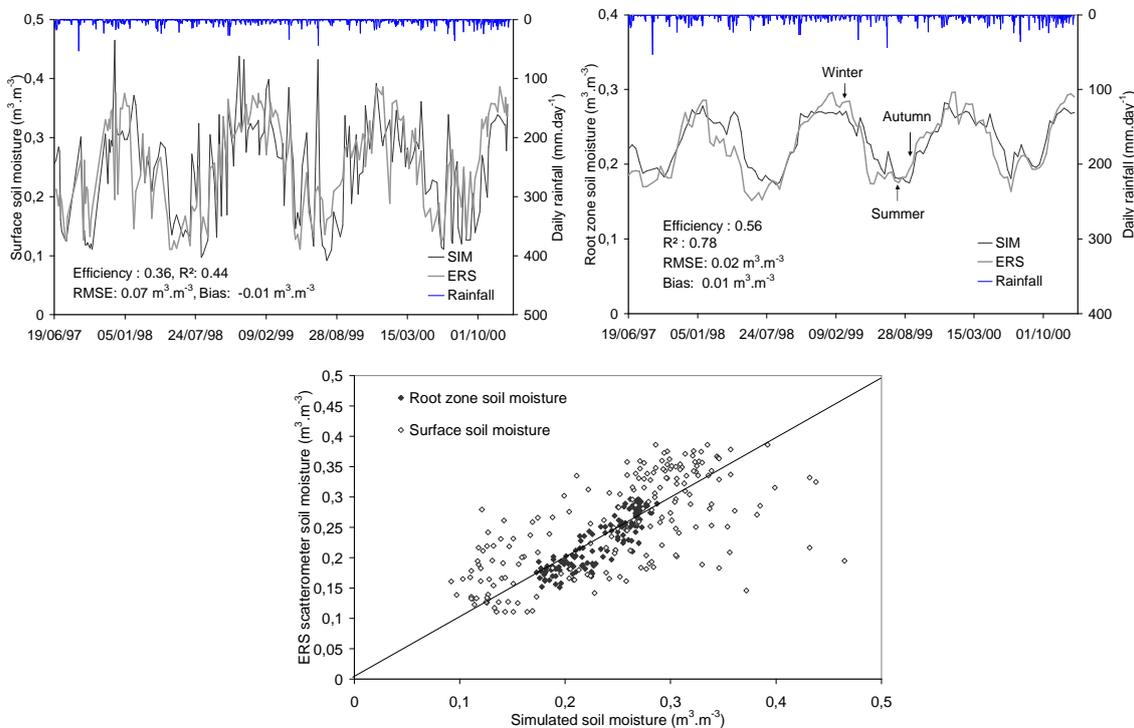
**Fig. 4.** Comparison of surface and root-zone soil moisture (m<sup>3</sup> m<sup>-3</sup>) for ERS scatterometer data (5 cm and 1 m depth, respectively) and simulation (1 cm and 1.5 m depth, respectively), from June 1997 to November 2000.
