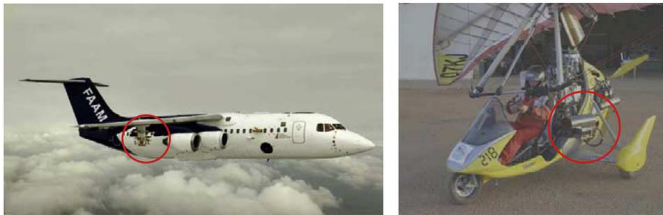
**Figure 4.** (left) FAAM BAe146 aircraft. The aerosol and cloud physics probes are visible mounted on the wing pylon as highlighted by the red circle. (right) ULA with the LAUVA lidar in horizontal pointing mode highlighted by the red circle.
