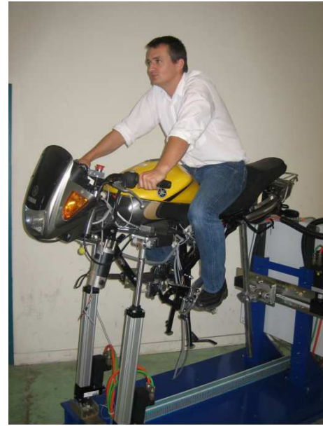
Fig. 6. Constructed riding motorcycle simulator
