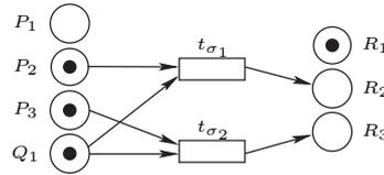
**Fig. 4.** Unfolded Petri net of high-level Petri net of Fig. 3-(a).
