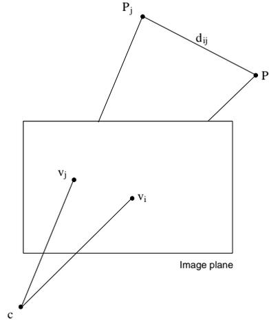
Fig. 2. Geometry of camera pose from points correspondences
