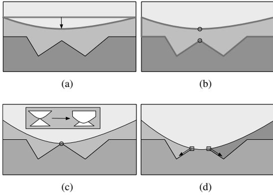
**Figure 14:** Erosion steps: (a) Erosion surface oversampling and vertices embedding update. (b) Research for the nearest collision. (c) Processing of the event according to the context, when a collision occurs (here, we assume that the erosion surface has some priority over the subsoil layer). (d) The erosion surface has eroded the layer: A new face is created and the contact vertices slide along the layer below.
