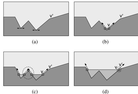
**Figure 11:** Sedimentation steps: (a) Searching for local minimums. (b) Creation of the first face and sliding of its extremities. (c) Creation of a new face and sliding of its extremities. Vertex  $v$  moves towards a vertex  $v'$  from the subsoil layer. (d) Merging of the two blocks and sliding of the new block extremities.  $v$  and  $v'$  collide, then  $v$  slides over  $v'$ .
