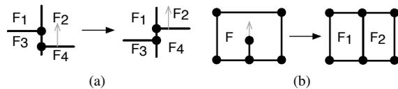
**Figure 2:** Examples of topological changes. (a) Vertex sliding over another vertex with topological changes of adjacency relationships between the four faces. (b) The vertex motion leads to split face  $F$  into  $F_1$  and  $F_2$ .
