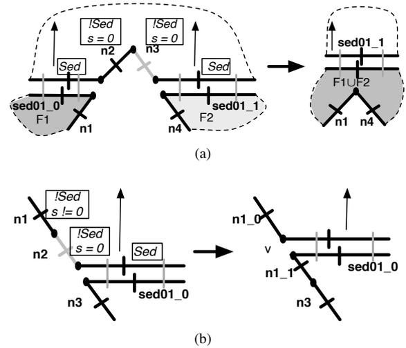
**Figure 12:** Collision sedimentation patterns (the current collision is shown in grey, predicates are framed): (a) Merging of two faces  $F1$  and  $F2$  coming from the same sedimentation process. (b) Sliding of a vertex over another vertex. Dashed lines represent a  $(\alpha_1 \alpha_0)^* \alpha_1$  link between two darts.
