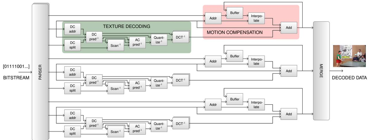
Fig. 1. MPEG-4 Simple Profile decoder description
