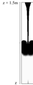
Figure 4. Sheared and resting zone when SCC is cast from the top of the formwork. In the black zone, the shear rate is greater than 0.1s^{-1} (from REF).
