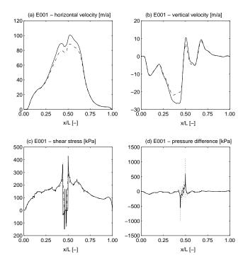
**Fig. 9.** Experiment E001 - (**a**) Horizontal surface velocity, (**b**) vertical surface velocity, (**c**) basal shear stress and (**d**) difference between the isotropic and hydrostatic pressure at the bed on mesh E\_1\_20 (dash-dot line), E\_20\_20 (dashed line) and E\_20\_20\_2nd (solid line).
