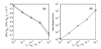
**Fig. 4.** (a) CPU time consumption (circle) and number of non-linear iterations  $N_{NL}$  (cross) relative to the reference run ( $\epsilon_L = 10^{-7}$ ) and (b) maximum of the relative difference with the reference run ( $\epsilon_L = 10^{-7}$ ) on the velocities as a function of  $\epsilon_L = \epsilon_{NL}/10$ , for experiment A with length  $L = 40 \, \mathrm{km}$ .
