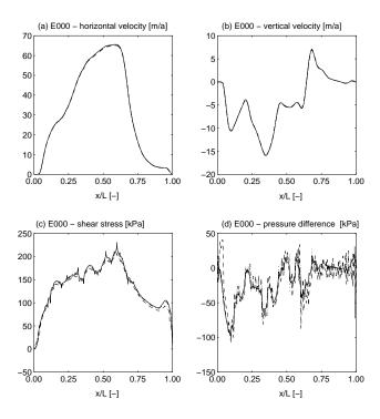
**Fig. 7.** Experiment E000 - **(a)** Horizontal surface velocity, **(b)** vertical surface velocity, **(c)** basal shear stress and **(d)** difference between the isotropic and hydrostatic pressure at the bed on mesh E\_1\_20 (dash-dot line), E\_unstruct (dotted line), E\_20\_20 (dashed line) and E\_20\_20\_2nd (solid line).
