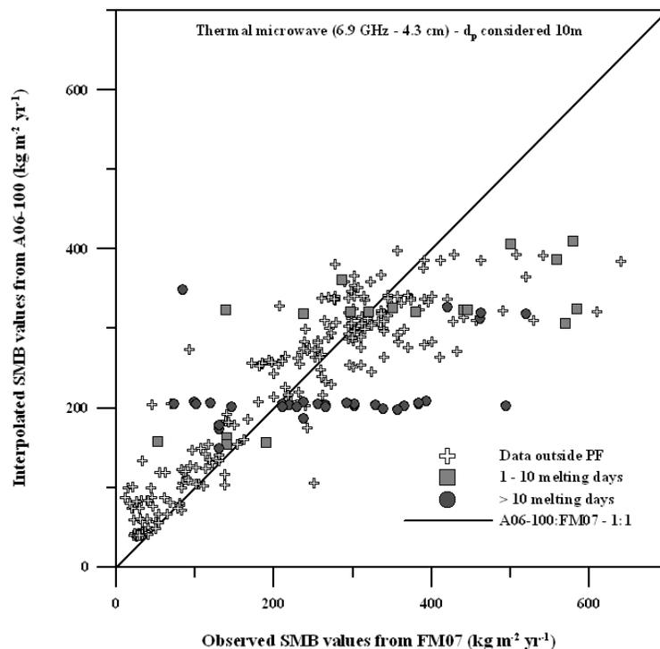
**Fig. 3.** Comparison between observed SMB values from filtered observational SMB data sets (M07) and interpolated SMB values averaged in 100 km resolution (A06-100) with distribution pattern of observed SMB points located in **Percolation Facies (PF)** ~melting events) areas. Cumulative melting days are calculated on the basis of 6.9 GHz microwave penetration depth ( $d_p$ ) of 10 m. SMB values are expressed in  $\text{kg m}^{-2} \text{yr}^{-1}$  (i.e. mm W.E.).
