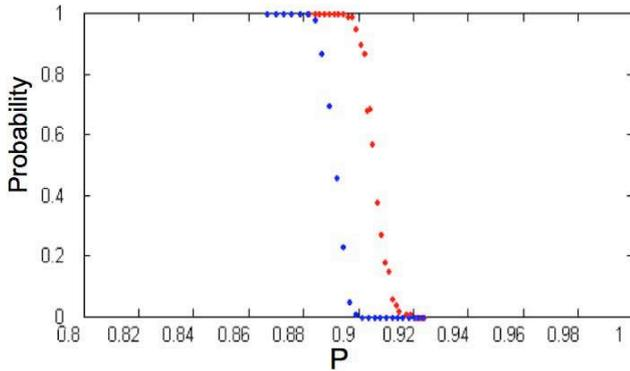
**Fig. 9.** This shows the effect of varying the vesicularity on the void (magma) percolation probability in the horizontal and vertical directions on a finite  $200^3$  lattice (100 simulations for each  $P$ ). With  $H_z=0.2$  blue and red correspond respectively to vertical and horizontal percolation thresholds.
