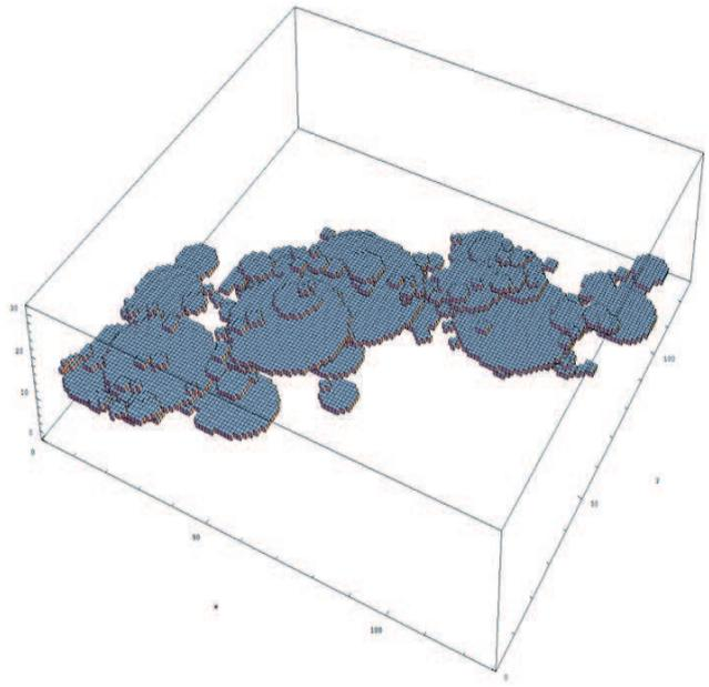
**Fig. 8c.** The percolating cluster from the realization shown in Fig. 8b. Although only a relatively thin layer of disks participate in the percolating cluster, the possibility of connecting in the vertical direction is enough to reduce the bubble percolation threshold  $P_c$  well below the 2-D value  $\approx 0.6$  (which we would obtain in the limit of planar disks infinitely thin in the  $z$ -direction).
