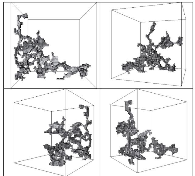
**Fig. 2c.** Four different view angles showing a simulation of the percolating magma cluster (largest magma fragment – in grey) with power law bubble distribution ( $B_3=0.85$ ) on a  $64^3$  simulation showing the extremely fragile and complex created structures at such high vesicularity ( $P=0.95$ ).
