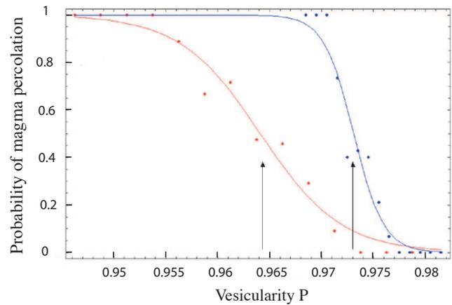
**Fig. 3b.** Same as Fig. 3a except for magma percolation.  $P_{3c,m}=0.973, 0.964$  for the power law (blue) and monodisperse (red) respectively bubbles. There were about 120 simulations in each case. Again the monodisperse value is slightly different from the literature (infinite) system value due to finite size effects.
