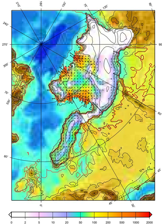
**Fig. 5.** Horizontal ice velocity of experiment MI 89 kyr BP, close to the maximum ice volume. Kara sea is covered by a high slow moving ice dome. Barents Sea presents large ice streams in the topographic troughs.
