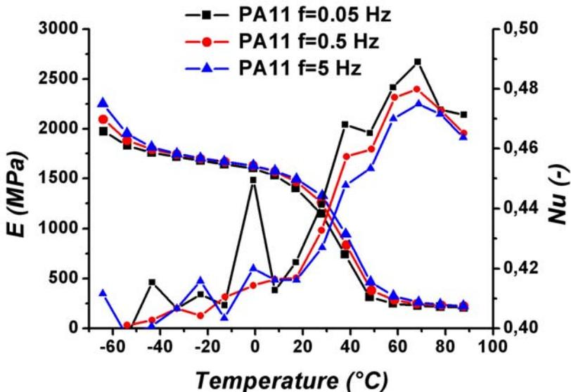
Fig. 1: Young Modulus (MPa) and Poisson ratio (-) evolution in function of the temperature
