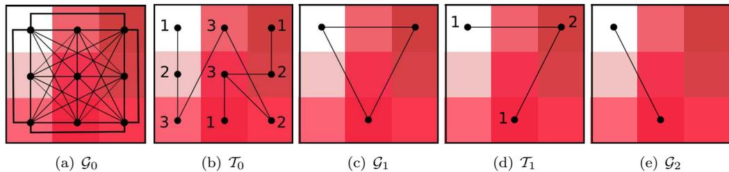
Fig. 2. The graphs  $\mathcal{G}_i$  and  $\mathcal{T}_i$  in the different steps of the algorithm for Hamiltonian path bounds extraction. For each  $\mathcal{T}_i$ , the vertices degrees are superimposed.  $\mathcal{T}_2$  is not shown here.
