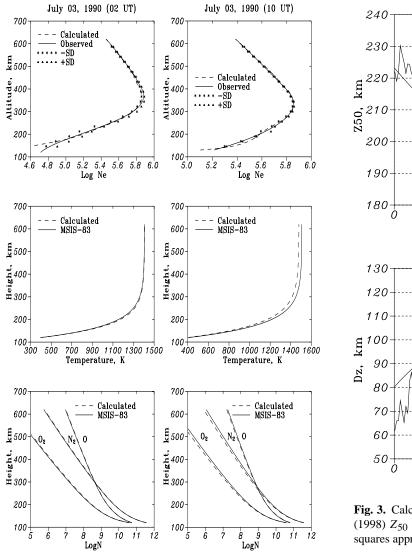
**Fig. 2.** Observed (together with a band of standard deviations) and calculated  $N_e(h)$  profiles for two UT moments (top panel). Calculated along with MSIS-83  $T_n$ , O, O<sub>2</sub>, and N<sub>2</sub> height profiles (middle and bottom panels).
