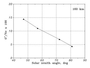
**Fig. 8.** Calculated dependence of the O<sup>+</sup>/Ne ratio on the solar zenith angle at a fixed (160 km) height.
