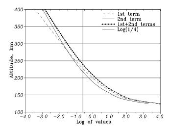
**Fig. 7.** Comparison of the two terms from the expression (3). Vertical line corresponding to  $\log_{10}(1/4)$  (see (4)) divides the ionosphere by the lower and the upper parts where molecular and atomic ions dominate.
