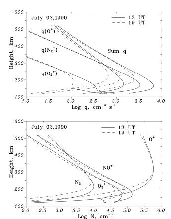
**Fig. 9.** Calculated height profiles of photo-ionization rates and corresponding ion concentrations for daytime (13 UT) and evening (19 UT) hours. Note the strong decrease in the photo-ionization rates at lower heights in the evening.
