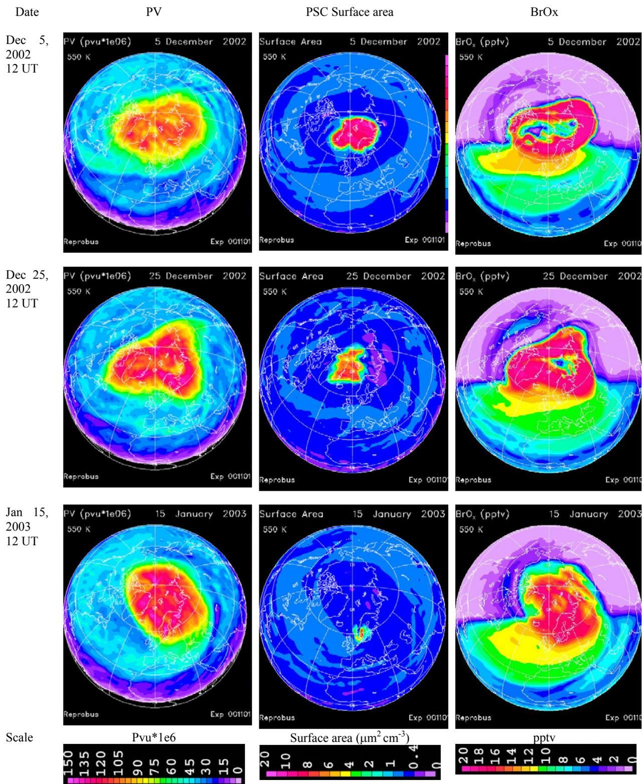
**Fig. 6a.** Vortex, PSC surface area and BrO<sub>x</sub> from REPROBUS at 550 K. Top panel: 5 December 2002. Middle panel: 25 December 2002. Bottom panel: 15 January 2003.
