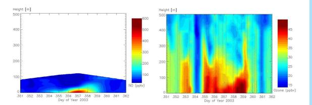
**Fig. 11.** Comparison of the vertical distribution of NO (left) and ozone (right) during Dec. 2003 at South Pole. These data are from concurrent vertical profile measurements of NO and ozone using a tethered balloon. (Figures adapted from Helmig et al., 2007a, 2007e).
