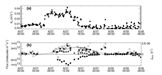
**Fig. 4.** (a) Eddy diffusivity measurements and (b) calculated fluxes (flux-gradient approach) during 27–28 June at Summit, Greenland. circles =  $NO_x$ , triangles = HONO, squares =  $HNO_3$ , solid line =  $J(NO_3^-)$ . Positive values indicate an upward flux. (Reprinted from Honrath et al., Vertical fluxes of  $NO_x$ , HONO and  $HNO_3$  above the snowpack at Summit, Greenland, Atmospheric Environment, 36, 2629–2640, 2002, with permission from Elsevier).
