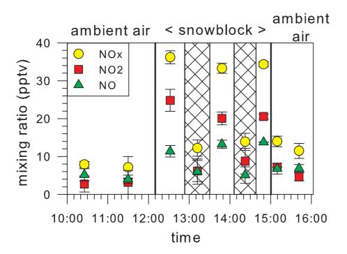
**Fig. 3.** Measurements of NO,  $NO_2$  and  $NO_x$  in a snowblock shading experiment at Neumayer Station, Antarctica (Jones et al., 2000). The first and final sections are measurements made in ambient air. Middle sections are measurements made within the snowblock, alternatively fully exposed to sunlight and fully shaded to eliminate any photochemical activity. Periods of shading are indicated by cross-hatching.
