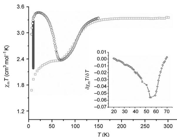
Figure 7. Plot of experimental  $\chi_m T$  versus  $T$  (squares) and temperature dependence of the product  $\chi_m T$  after LIESST (circles), in the 6–300 K range for compound **2**. The inset shows the derivative of the product  $\chi_m T$  with a  $T(\text{LIESST})=54 \text{ K}$ .
