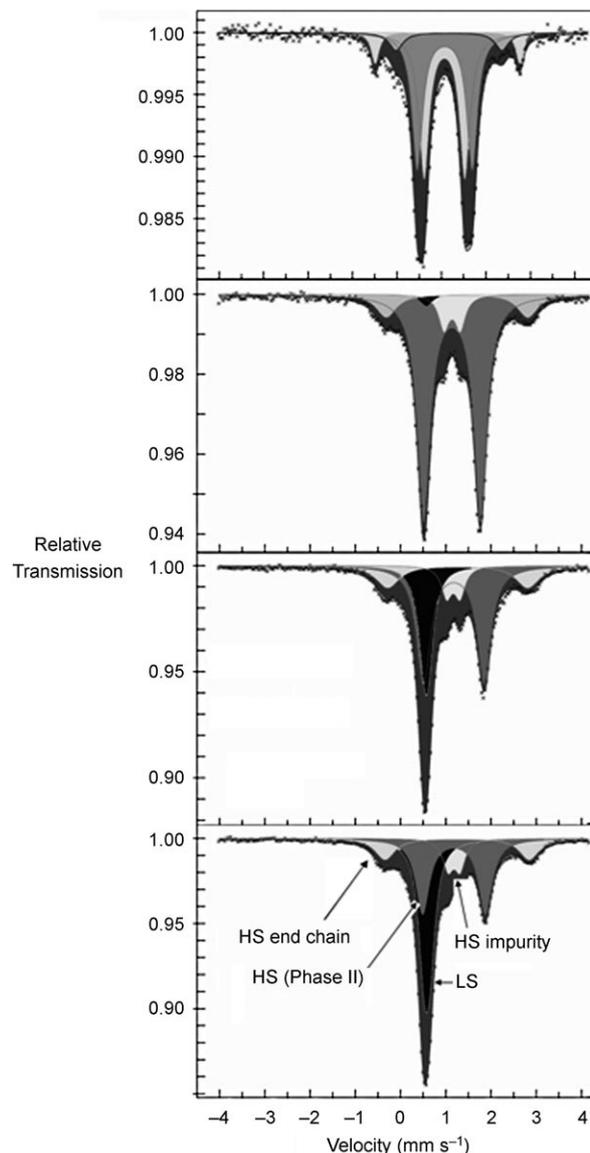
Figure 9. Mössbauer spectra for compound **2**. From top to bottom: 297, 175, 110 and 80 K. Parameters are given in Table 5.
