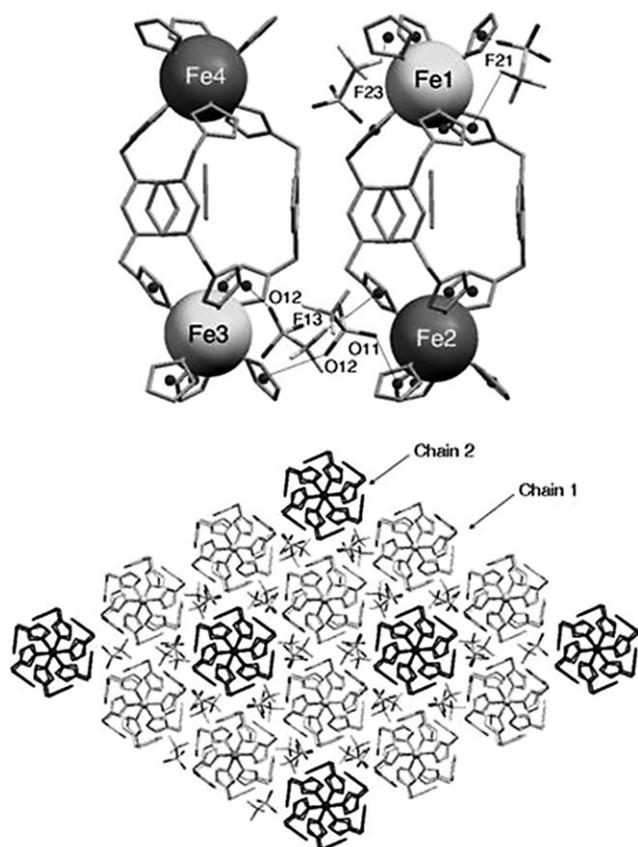
Figure 4. Top: Anion- $\pi$  interactions occurring in chain1 and chain2 in compound **2**. All tetrazoles involved in anion- $\pi$  interactions are marked with their centroids. Bottom: View of the packing along the  $c$  axis for compound **2**.
