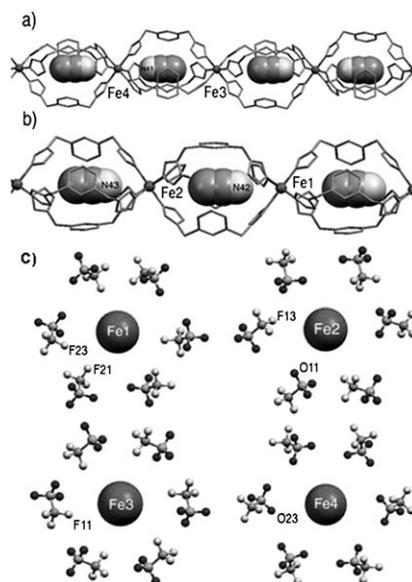
Figure 3. View along the  $b$  axis of the two crystallographically independent chains, showing the orientation of the trapped solvent molecules in a) Chain2 and b) Chain1 of compound **2**. c) View of the different anion-surroundings for each of the four independent Fe<sup>II</sup> centres present in compound **2**, all depicted independently and viewed along the  $c$  axis.
