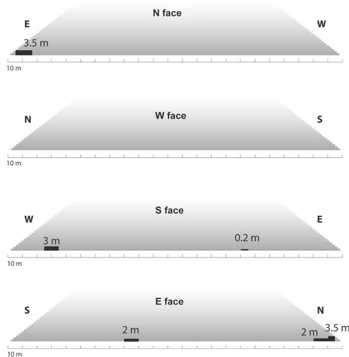
Figure 16. Kheops Pyramid. Localization of the visible outcrops of the original hill.
