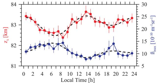
**Fig. 3.** Diurnal variation of NLC altitude (red circles) and brightness (blue circles) above ALOMAR for the integrated data set from 1997 to 2003. Only clouds brighter than  $\beta_{max} > 4 \times 10^{-10} \text{ m}^{-1} \text{ sr}^{-1}$  are included. The vertical bars represent the 95% significance limits of the hourly mean values, and the dashed curves are harmonic fits to the data.
