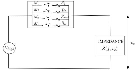
Fig. 3: Vdd-hopping, voltage supply and load
