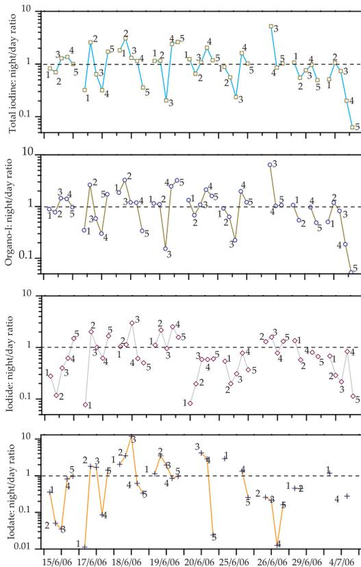
**Fig. 2.** Size segregated iodine concentrations from nighttime samples divided by iodine concentrations in samples from the previous day. Numbers indicated impactor stage (i.e. aerosol size fraction) and the dotted line shows 1:1 relationship between day and night. Note that were no data exists either measurement was not possible or concentrations were below the detection limit.
