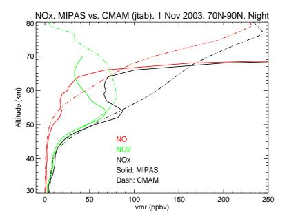
**Fig. 7.** Mean NO,  $NO_2$ , and  $NO_x$  profiles for the Northern Hemisphere polar cap (70–90° N) at nighttime conditions for the 1 November 2003 measured by MIPAS and modeled by the CMAM model.
