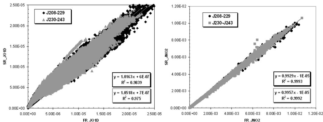
**Fig. 15.** (a): Correlation plot for  $j\text{-}(O^1D)$  measured using the University of Leicester's filter radiometer (FR) and diode array spectroradiometer (SR). (b): Correlation plot for  $j\text{-}(NO_2)$  measured using the University of Leicester's filter radiometer (FR) and diode array spectroradiometer (SR). The two Julian day ranges refer to data from the first and second halves of the campaign, respectively.
