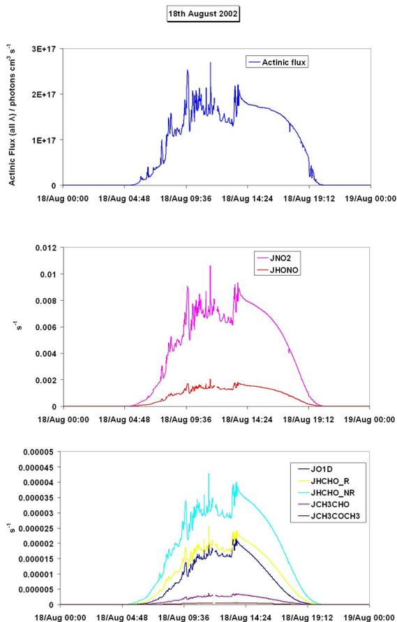
**Fig. 16.** (a): Actinic flux, (b):  $j(\text{NO}_2)$  and  $j(\text{HONO})$ , (c):  $j(\text{O}_1\text{D})$ ,  $j(\text{HCHO})_{\text{NR}}$  (non-radical,  $\text{HCHO} + h\nu \rightarrow \text{H}_2 + \text{CO}$ ),  $j(\text{HCHO})_{\text{R}}$  (radical,  $\text{HCHO} + h\nu \rightarrow \text{HCO} + \text{H} \rightarrow \text{HO}_2 + \text{HO}_2 + \text{CO}$ ),  $j(\text{CH}_3\text{CHO})$ , and  $j(\text{CH}_3\text{COCH}_3)$  for a clean day 18 August 2002.
