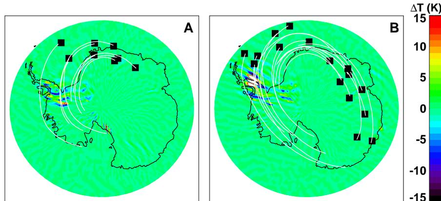
**Fig. 4.** Color-coded MWF3 hindcast mountain-wave temperature perturbations for 12:00 UT on 10 June (A) and 12:00 UT on 11 June (B). Overlaid backward trajectories (white lines) start at the times and locations of MIPAS NAT observations (squares) on 11 June (A) and 12 June (B) and end at 00:00 UT on 10 June (A) and 00:00 UT on 11 June (B). Note that the MWF2 solutions in Fig. 3 show peak wave amplitudes only, whereas the MWF3 runs in this figure provide both amplitude and phase.
