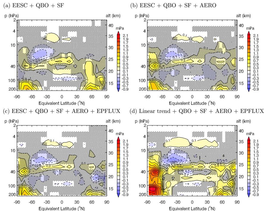
**Fig. 10.** Vertical cross-section of the mean ozone partial pressure residuals 1996–2004 for different model versions fitted to period January 1979 to December 1995. **(a)** Model including the effects of EESC, QBO and solar cycle only. **(b)** Same as (a) but including the effect of volcanic eruptions. **(c)** Same as (b) but including effect of Eliassen-Palm flux. **(d)** Same as (c) but fitting a linear trend instead of EESC.
