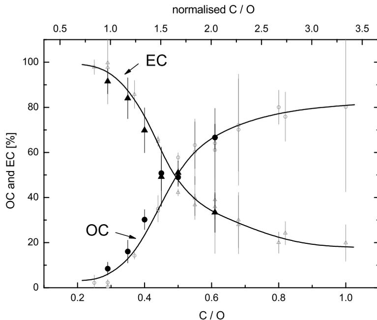
**Fig. 1.** Dependence of the particle composition (OC and EC content) on the C/O atomic ratio in the burner. Full symbols indicate measurements on samples from the NAUA chamber, open symbols indicate samples taken directly behind the CAST burner. The upper scale gives the C/O ratio normalised to the stoichiometric ratio of 0.3. The stoichiometric ratio separates fuel-lean (normalised C/O ratio <1.0) and fuel-rich (normalised C/O ratio >1) burner conditions.
