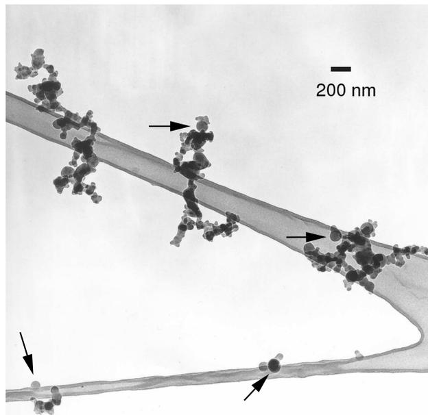
**Fig. 3.** TEM image showing the morphologies of carbonaceous aerosol particles produced at  $C/O=0.45$ . The arrows indicate larger spherical particles either isolated or attached to the soot aggregates.
