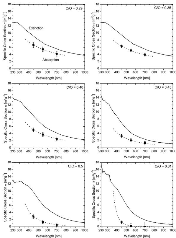
**Fig. 5.** Specific extinction (solid lines) and absorption (squares) cross sections derived for NAUA aerosol samples produced at different C/O ratios. The absorption values originate from extinction and total scattering (nephelometer) measurements (difference method, see Sect. 1). Dashed lines represent power laws fitted through the measured absorption cross sections.
