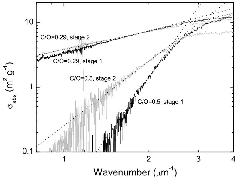
**Fig. 7.** Double logarithmic representation of the absorption behaviour in the visual range for samples produced at C/O ratios of 0.29 and 0.50 and deposited on impactor stages 1 and 2. The figure shows that the power-law behavior is no longer valid at wavenumbers larger than  $2.5 \mu\text{m}^{-1}$ .
