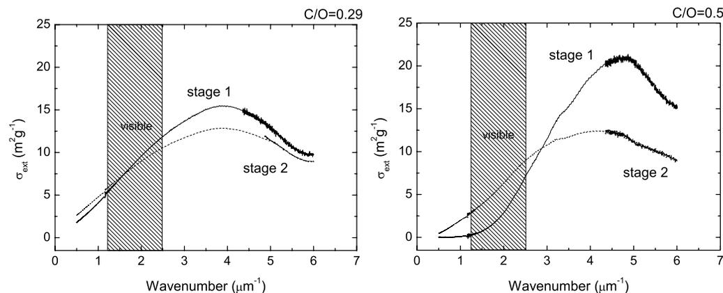
**Fig. 8.** Specific extinction cross sections corresponding to the samples produced with C/O ratios of 0.29 and 0.50 and deposited at the impactor stages 1 and 2. The smooth (noisy) traces represent measurements with the UV-VIS spectrometer (the VUV spectrometer). The combined spectra reveal the presence of a prominent band with a maximum in the  $3\text{--}5\ \mu\text{m}^{-1}$  range. The visual range where the Ångström exponent was determined is shaded.
