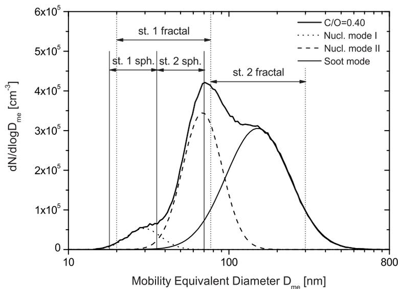
**Fig. 2.** Number size distribution measured by SMPS for an aerosol produced by the CAST at C/O=0.40. The vertical lines indicate the size ranges deposited on impactor stages 1 and 2 for the cases of compact spherical particles and fractal aggregates, respectively (see Sect. 4.1).
