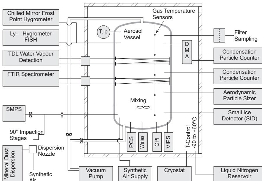
**Fig. 1.** Schematic of the AIDA (Aerosol Interaction and Dynamics in the Atmosphere) aerosol chamber with instrumentation for heterogeneous ice nucleation studies of mineral dust aerosols at simulated cloud conditions.
