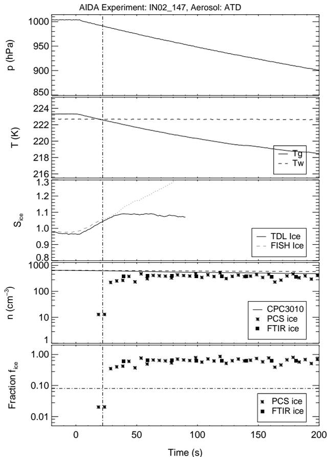
**Fig. 5.** Time series from experiment IN02\_147 with ATD at 223.3 K. Panel 1 (from top): pressure; panel 2: mean gas temperature; panel 3: ice saturation ratio; panel 4: number concentration of aerosol and ice particles (see text); panel 5: ice particle fraction to total aerosol. The vertical dashed-dotted line marks the time when the ice-activated fraction  $f_i$  exceeded a value of 0.08.
