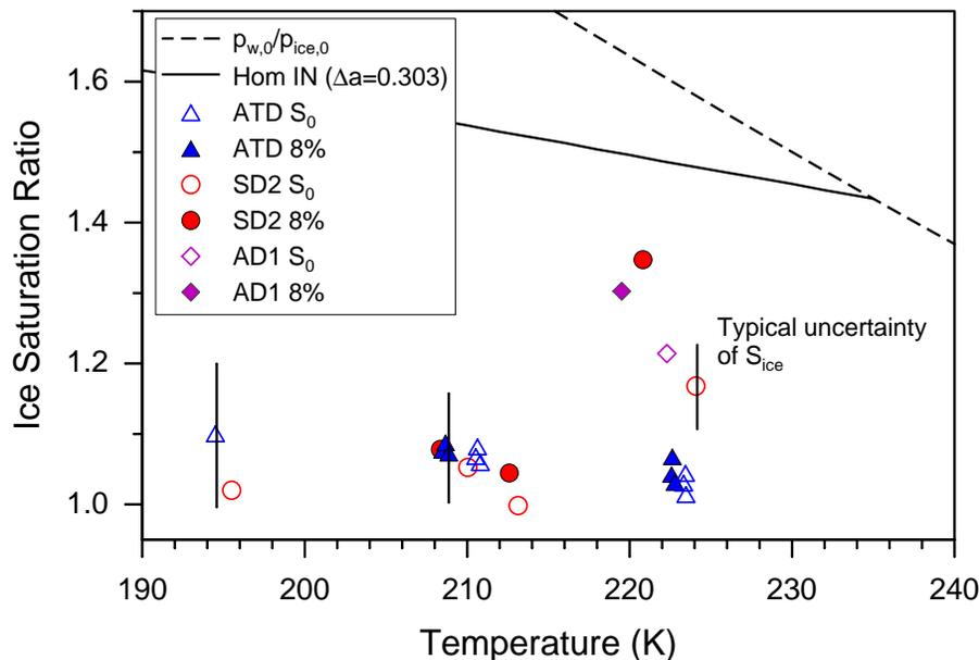
**Fig. 9.** Threshold ice saturation ratios for freezing onset (open symbols) and for 8% ice activated aerosol fraction (filled symbols). The vertical bars show the estimated uncertainty for  $S_i$ . Also shown are the ratio of the saturation pressures for pure liquid water (dashed line) and typical ice saturation ratios for the freezing of solution droplets according to Koop et al. (2000). The water vapour saturation pressures are taken from Murphy and Koop (2005).
