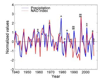
**Fig. 13.** Inter-annual variability of the mean winter (NDJFM) precipitation at S. Julião Tojal (solid curve), and the corresponding winter NAO index, multiplied by -1 to facilitate analysis (dashed curve); both curves have been normalised and so are dimensionless (period 1932–2007). Diamonds – events of shallow landslides activity; Triangles – events of deep landslides activity.
