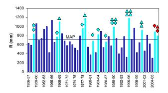
**Fig. 3.** Annual precipitation (climatological year) distribution at S. Julião do Tojal (reference rain-gauge) and landslide incidence from 1956/1957 to 2006/2007. MAP – Mean Annual Precipitation (723 mm). Light blue bars – years with landslide activity; Diamonds – events of shallow landslides activity; Triangles – events of deep landslides activity. Landslide events occurred in 2006 are marked in red.
