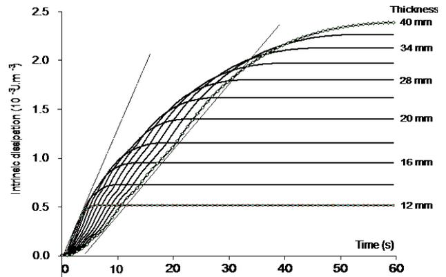
**Figure 7:** Change of the intrinsic dissipation with time at the outer surface for several tube thicknesses
