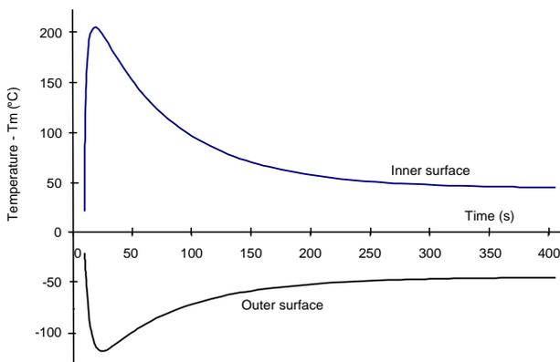
**Figure 3:** Temperature minus average temperature change versus time in the tube (thickness 15 mm)
