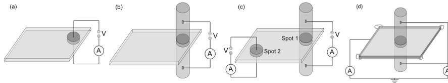
**Fig. 1.** Different ways to measure electrical conductivity. **(a):** Standard procedure, no load; **(b):** under load; **(c):** measuring at two places, one under load; **(d):** measuring a battery current.
