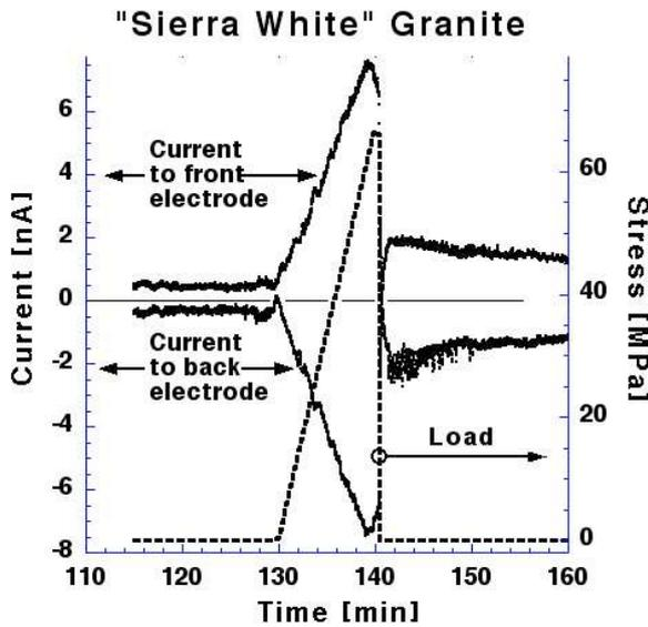
**Fig. 4.** As one end of the granite slab is loaded (dotted line) electrons flow out of the stressed rock volume to ground (lower curve) and from ground into the unstressed rock (upper curve). The two currents are legs of one and the same circuit.
