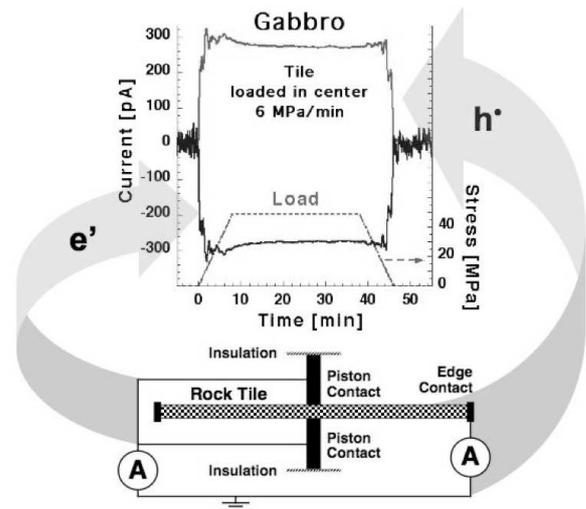
**Fig. 5.** Outflow currents from a gabbro tile,  $30 \times 30 \times 1 \text{ cm}^3$ , loaded at the center ( $\sim 10 \text{ cm}^3$ ) from 0 to 48 MPa and kept at constant load for 30 min. Currents increase rapidly at beginning, reach a steady state value and decay slowly. Upon unloading currents return to zero.
