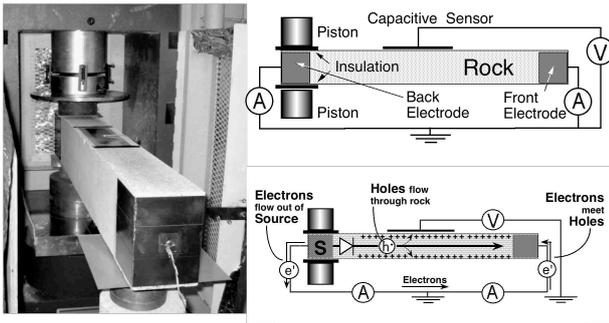
**Fig. 3.** Experimental set-up with a slab of granite, one end in a press, Cu contacts attached to front and the back (left); electric circuit with ammeters to measure currents, one between each Cu contact and ground, capacitive sensor to measure the surface charge (upper right); circuit showing the flow of electrons through the outer circuit and the flow of holes through the rock (lower right).
