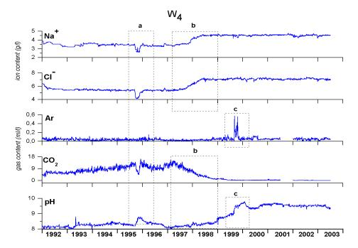
**Fig. 2.** Time-series of Na<sup>+</sup> and Cl<sup>-</sup> ion contents, of Ar and CO<sub>2</sub> gas contents and of pH value at W<sub>4</sub> from 1 January 1992 to 30 June 2003. Clear disturbances stand up in 1995–1996 (period a), in 1997–1998 (period b) and in 1999–2000 (period c).
