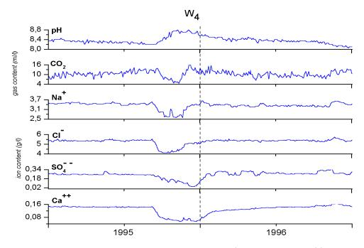
**Fig. 3.** From the top to the bottom, the pH value, the CO<sub>2</sub> gas content and the Na<sup>+</sup>, Cl<sup>-</sup>, SO<sub>4</sub><sup>--</sup> and Ca<sup>++</sup> ion contents at W<sub>4</sub> from 1 January 1995 to 31 December 1996. The vertical line indicates the occurrence of the 1 January 1996 earthquake (M=6.9) and the beginning of the Karymsky volcano eruption.
