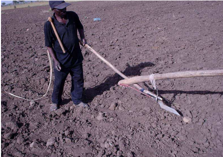
Fig. 4. Maresha modified Subsoiler.
