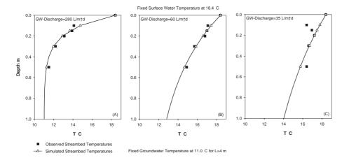
**Fig. 6.** Comparison of observed and simulated streambed temperatures for three example profiles. The illustrated profiles represent high **(a)**, medium **(b)** and low **(c)** groundwater discharges and are located proximal to the positions of streambed piezometers P5 (a), P4 (b) and P1 (c).
